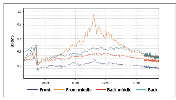
Figure 5 - Vibration intensity levels (RMS) versus time for four measurement sensors. The higher intensity top (orange) trace was linked to a plugged spray nozzle causing non-uniform coating adjacent to this sensor.
