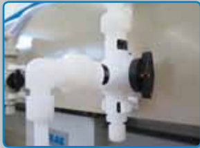
3 way valve for calibration and dip tray for measuring jar
